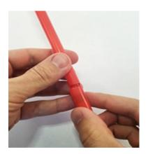
5) Squeeze the straw where the battery is, and the LED should light up. Slide the longer piece over the one and wrap with electrical tape. Squeeze the handle to light up your lightsaber!
