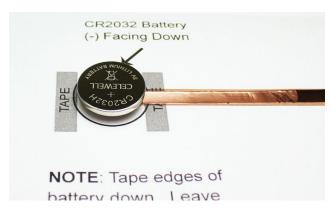
**NOTE:** Make sure to leave the middle exposed so the circuit can contact it.
